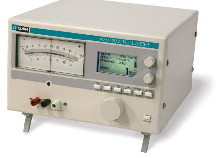
the instrument. It continuously displays the status of the primary selected parameters and mode of operation. The current range setting is shown in large bold numbers to eliminate range reading errors incurred when reading knob position.
